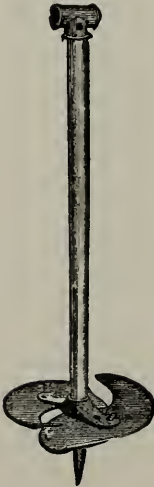
FIG. 266. AUGER FOR BORING HOLES IN THE GROUND TO PLACE FENCE POSTS IN.
