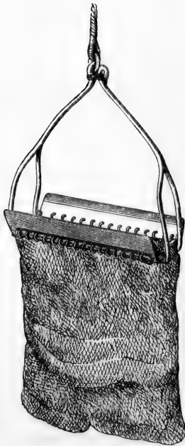
FIG. 200.—BALL DREDGE. (AFTER WYVILLE THOMSON.)
