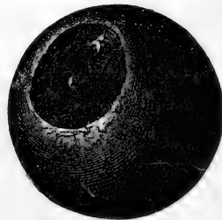
FIG. 160.—SPHERULE WITH METALLIC NUCLEUS COATED WITH BLACK MAGNETITE, SUPPOSED TO BE OF COSMIC ORIGIN ("CHALLENGER").
