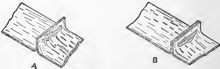
FIG. 52. BELT LACING WITH ENDS TURNED UP.
