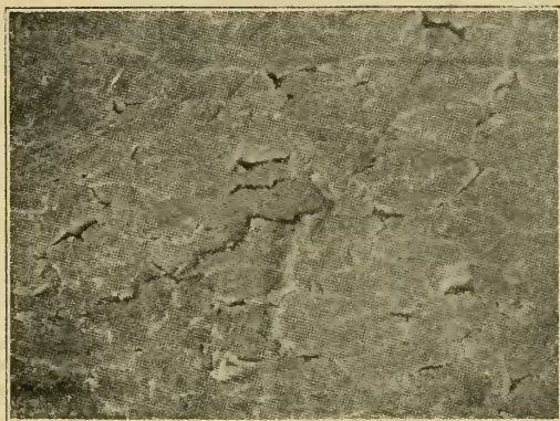
FIG. 31—ILLUSTRATION OF SEAMY COLOR AND ALSO OF LACK OF PRESSING
