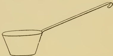
FIG. 6—THIS STYLE OF DIPPER HAS A SOLID HANDLE AND IS EASY TO KEEP CLEAN IN EVERY PART
