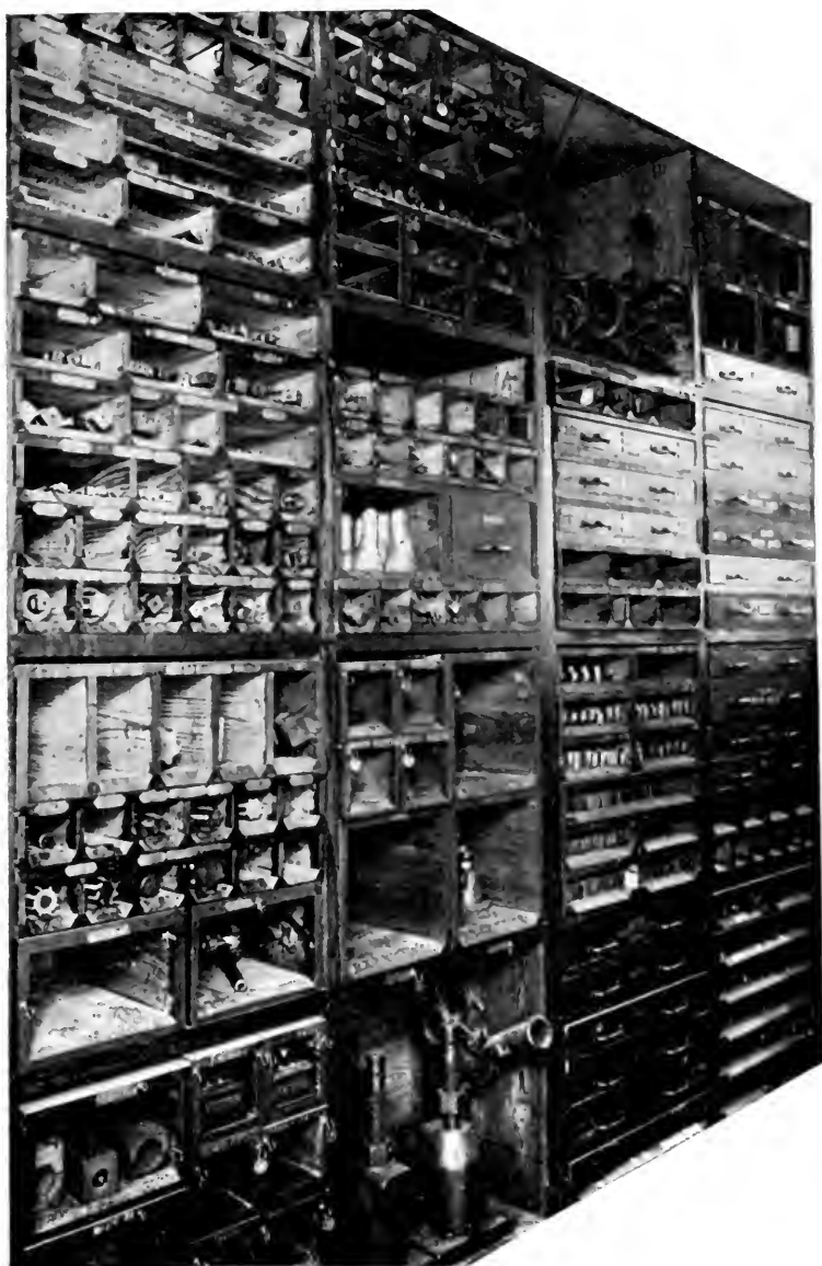
FIG. 3. — Rack for tools of various classes, having drawers for stocking milling cutters.
