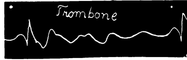
FIG. 5. WAVE FROM A LOW NOTE OF A TROMBONE. The whole curve between the sharp upper points is a single wave. \times 2,000 .
