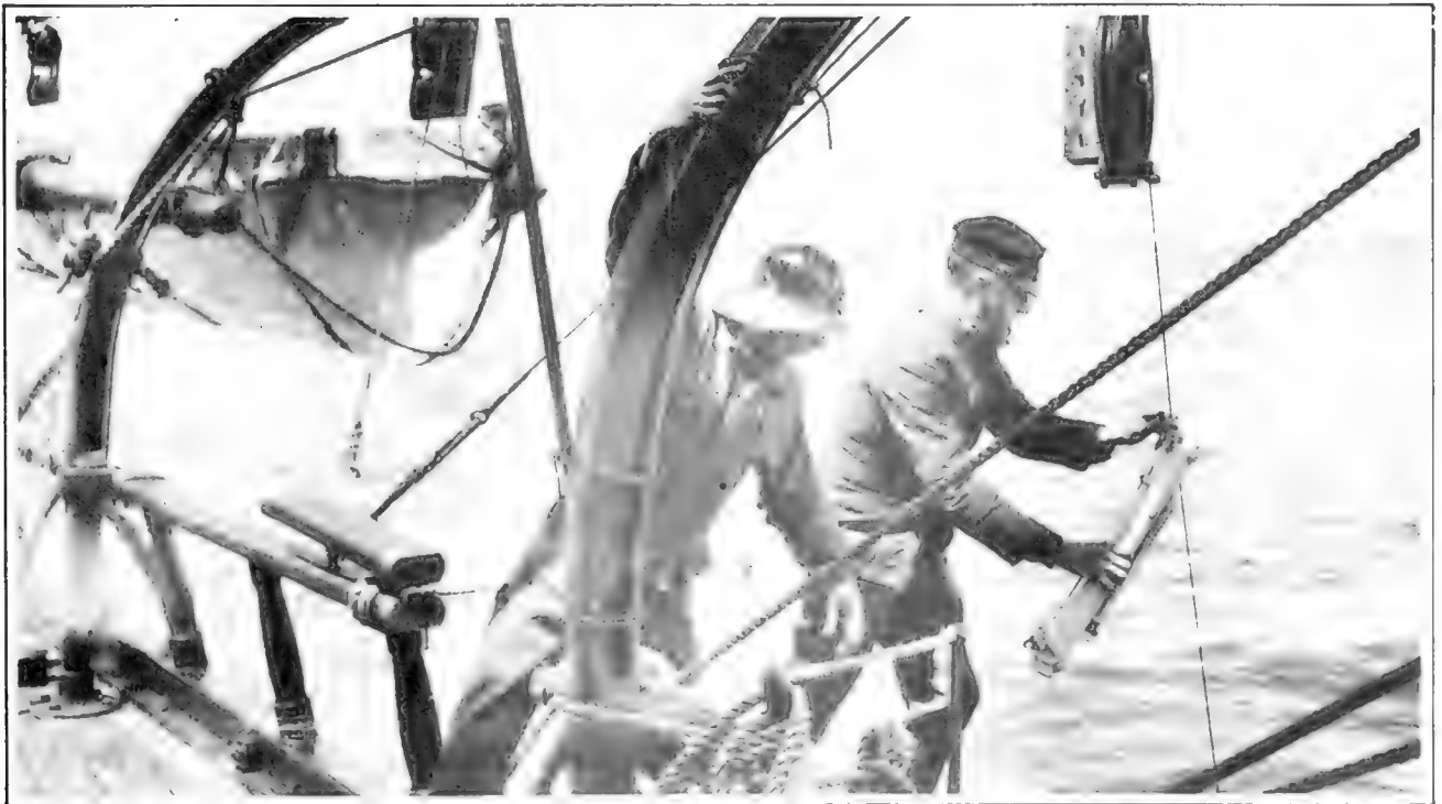
Fig. 22. Captain Ault about to remove a "Nansen bottle" which contains a sample of sea water obtained from the deep. The thermometers attached to the bottle give the temperature at the level at which the bottle was reversed
