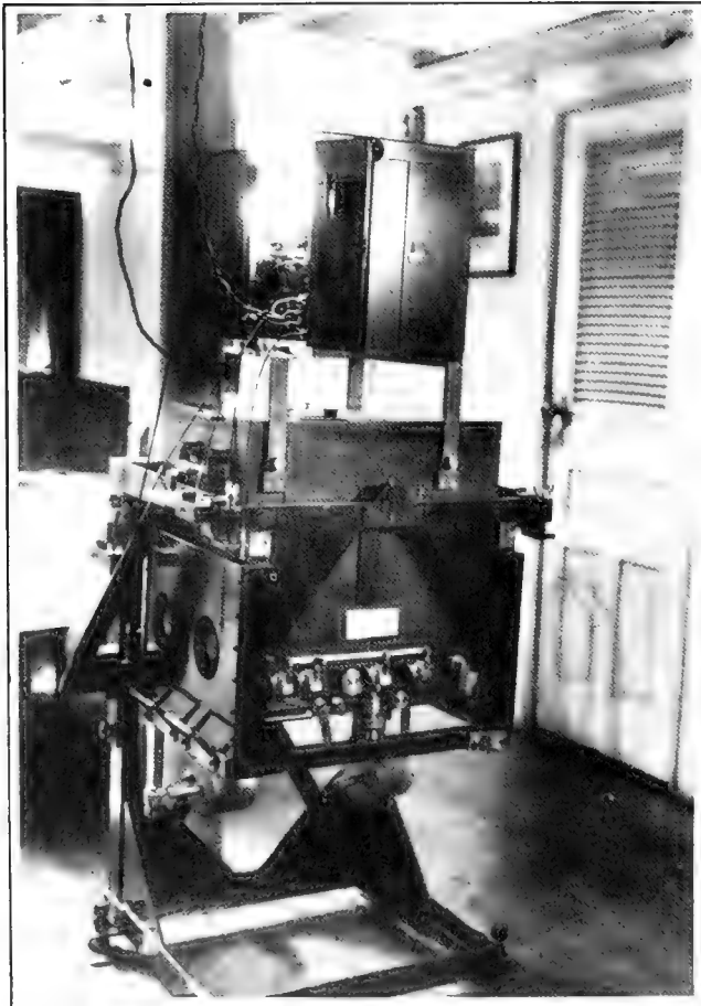
Fig. 33. Pendulum apparatus installed in the cabin for measuring the force of gravity
