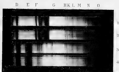
NEODYMIUM AMMONIUM NITRATE 1 AT 20° C. 2 AT 100° C. PRASEODYMIUM AMMONIUM NITRATE 3 AT 20° C. 4 AT 100° C.
