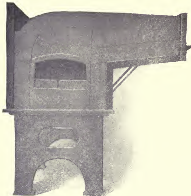
Furnace with front casting removed to show special shaped brick lining.
