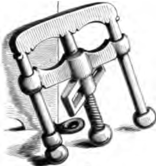
FIG. 3.—Thumb Screws with inner bars hollowed.
