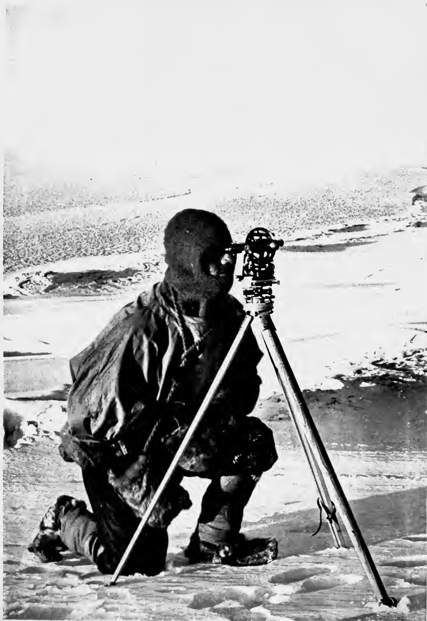
LIEUT. E. R. G. R. EVANS SURVEYING WITH THE FOUR-INCH THEODOLITE WHICH WAS USED TO LOCATE THE SOUTH POLE
