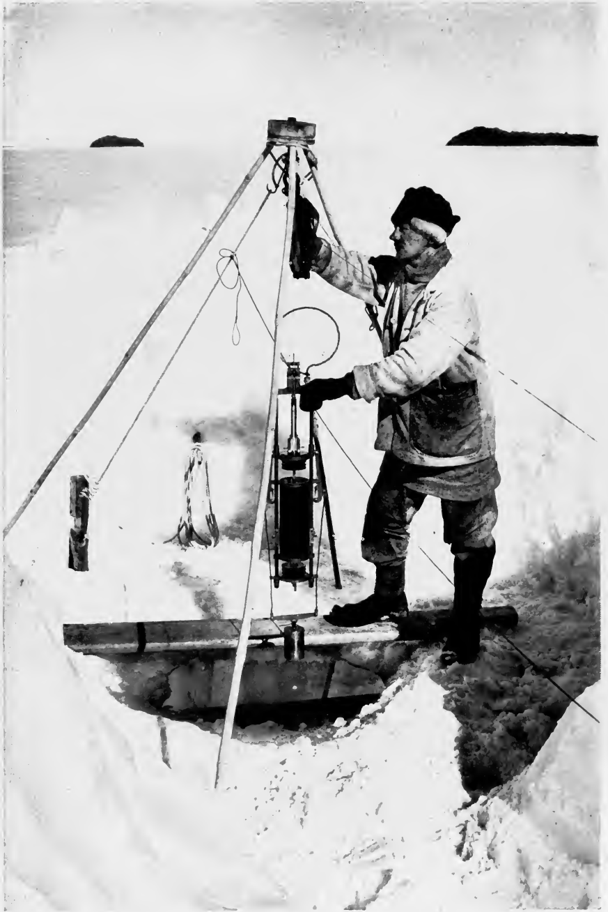
E. W. NELSON WITH THE NANSEN-PETERSEN INSULATED WATER-BOTTLE
