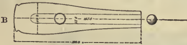
B.—The 15-inch Rodman of 1862. Length, 16 feet; weight, 20 tons; charge, 130 pounds; projectile, 450 pounds; muzzle energy, 9,000 foot tons.
