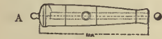
A.—The 42-pounder of 1812. Length, 10 feet; weight, 4 tons; charge, 10 pounds; projectile, 42 pounds; muzzle energy, 800 foot tons.
