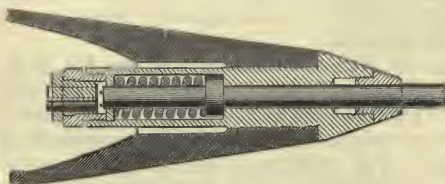
Percussion Lock and Firing-pin, Ericsson's Torpedo.
