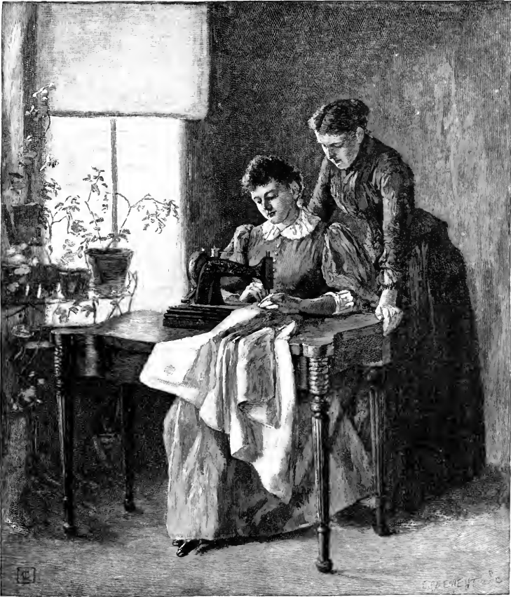
Sewing Machine Run by Electricity; the entire motor concealed in the wheel-case at the left.
