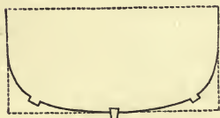
FIG. 77. Midship Section of Beach Boat.
