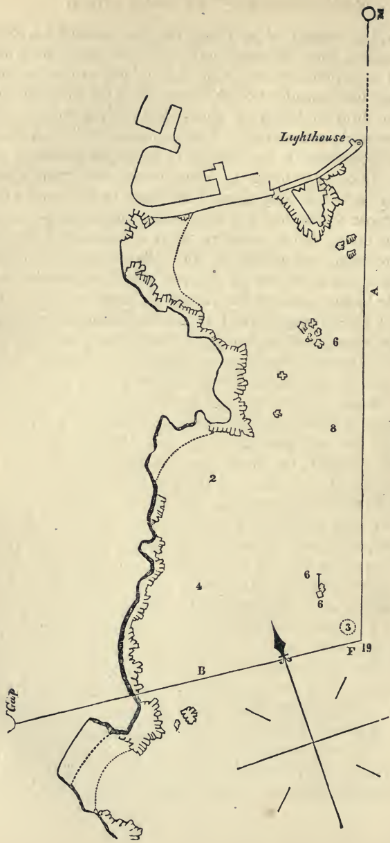
FIG. 1.—Chart of part of Guernsey, illustrating Marks and how to take them.
