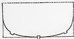
FIG. 77. Midship Section of Beach Boat.
