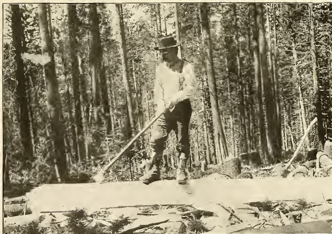
FIG. 2.—PEELING THE BARK FROM THE LODGEPOLE PINE. MAKING A TIE OUT OF LODGEPOLE PINE TIMBER, BOZEMAN, MONT
