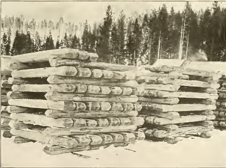
FIG. 2.—LODGEPOLE PINE PILED TO TEST INFLUENCE OF PREVAILING WINDS ON DRYING.
