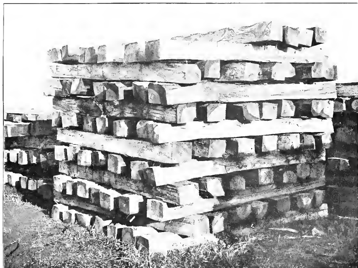
FIG. 2.—OAK PILES, SHOWING LOWEST TIER ON THE GROUND—A POOR METHOD.
