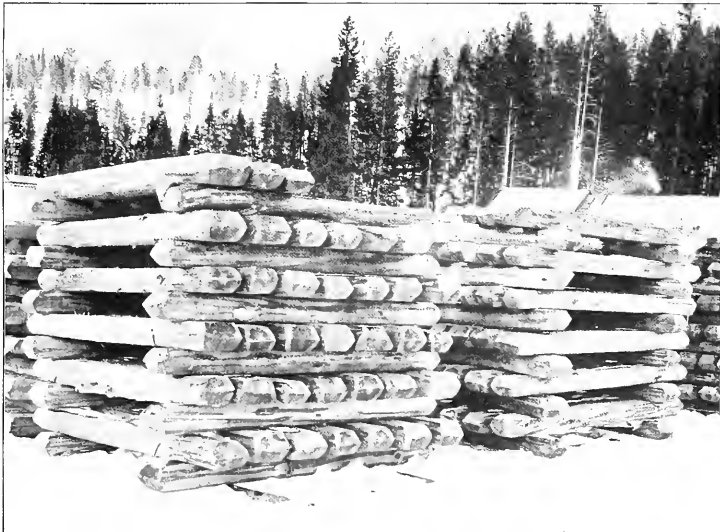
FIG. 2.—LOGS POILED TO TEST INFLUENCE OF PREVAILING WINDS ON DRYING.
