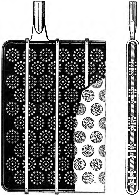
FIG. 43.—Lloyd's Perforated Sheet Protection.
