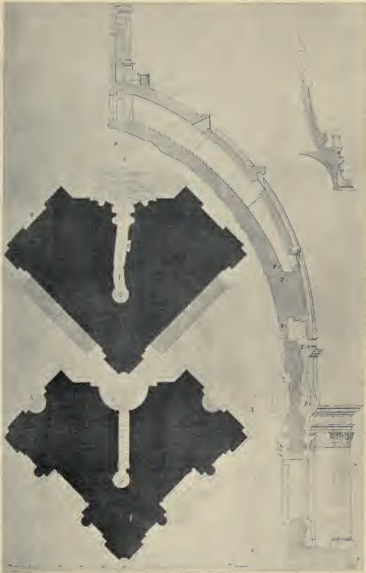
St. Peter's. Plan showing how the Dome and the Shrine Galleries of its piers are ascended.—From Pistolesi's "Il Vaticano."
