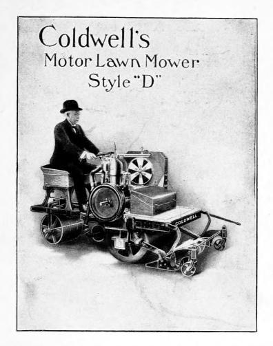
The machine weighs 2,000 pounds, and will negotiate 25 per cent. grades. It consumes from ½ to ¾ of a gallon of gasoline per hour, cuts a 40-inch swath, and will do three times as much work in a day as any ordinary horse lawn mower. Will almost pay for itself in a single season.
