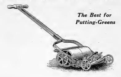
This mower is made to meet the demand for a machine that will more perfectly cut borders, verges, etc., and yet retain all the other features necessary in a mower for general work. The great advantage of this mower is the substitution of a bicycle chain for the gears generally used in this style of mower. This reduces the friction to a minimum. The machine with six blades is highly recommended by most of the leading golf clubs in America for work on putting-greens.
