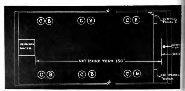
Plan for auditorium outlets. These outlets can be used for projection outside of booth for showings of films to small grou
