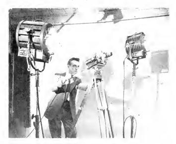
An Eastman Cine Special with synchronous motor is used for studio production at Ohio State University.
