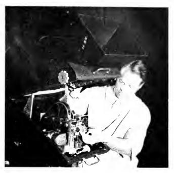
Above: 16mm aluminum blimp made by department for use with Cine Special camera; fits any tripod mount, also includes mercury switch and special lighting.
