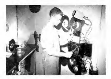
Iowa's A-V Bureau uses this 16mm motion picture printer for making duplicate prints as well as work prints of both picture and sound tracks for University films.
