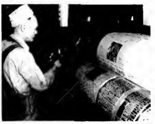
The molded plate with the story is on the press—ready to go into production.
