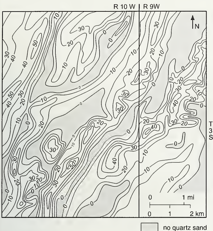
Figure 38 Map showing net sandstone thickness in the Big Clifty Sandstone in part of Gibson County, Indiana (modified from Specht 1985). Contour interval is 10 feet (3 m).
