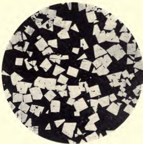
FIG. 2. ANTIMONY-TIN ALLOY WITH CRYSTALS OF Sb-Sn.
