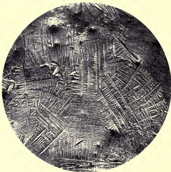
FIG. 1. DENDRITIC STRUCTURE OF ANTIMONY.
