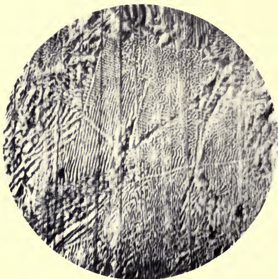
FIG. 2. EUTECTIC ALLOY OF BISMUTH AND TIN.
