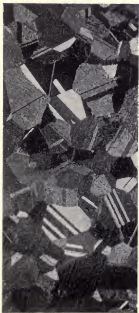
FIG. 3. ANNEALED BRASS— CRYSTALLINE STRUCTURE.
