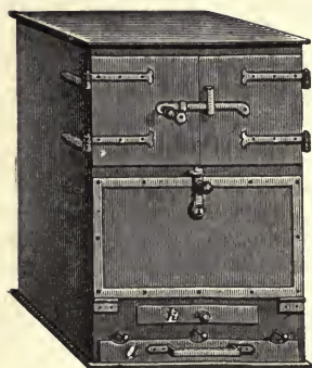
FIG. 32.—Two-stage coke stove.
