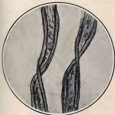
FIG. 87.— Cotton fibers magnified.
