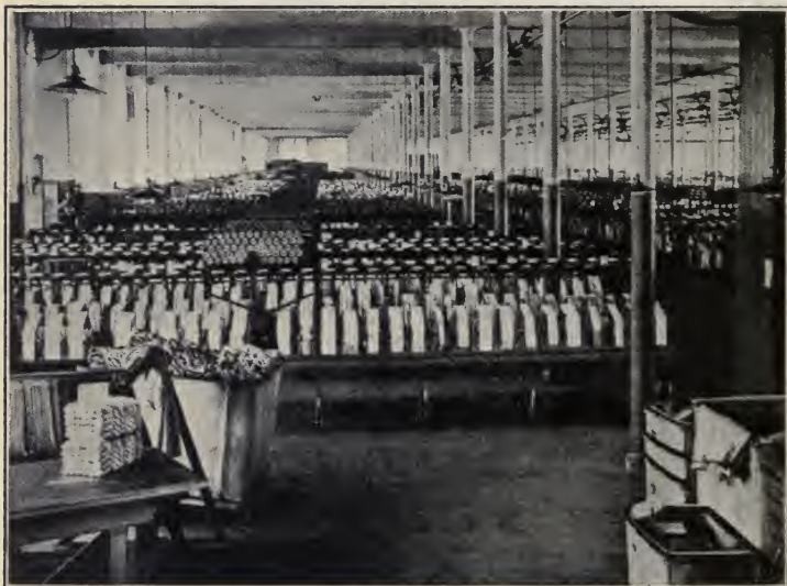
FIG. 82.—Winding room. Silk on swifts.
