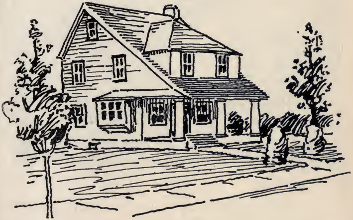
FIG. 9. — A modern small house with the "lean-to" motif. Notice that the long slope faces the front.
