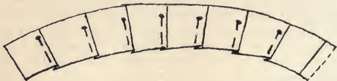
FIG. 139. — Lapping of slashed paper pattern for side crown. The method of lapping is the same for the brim.
