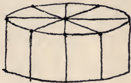
FIG. 147. — Square edged crown showing crossing of wires.
