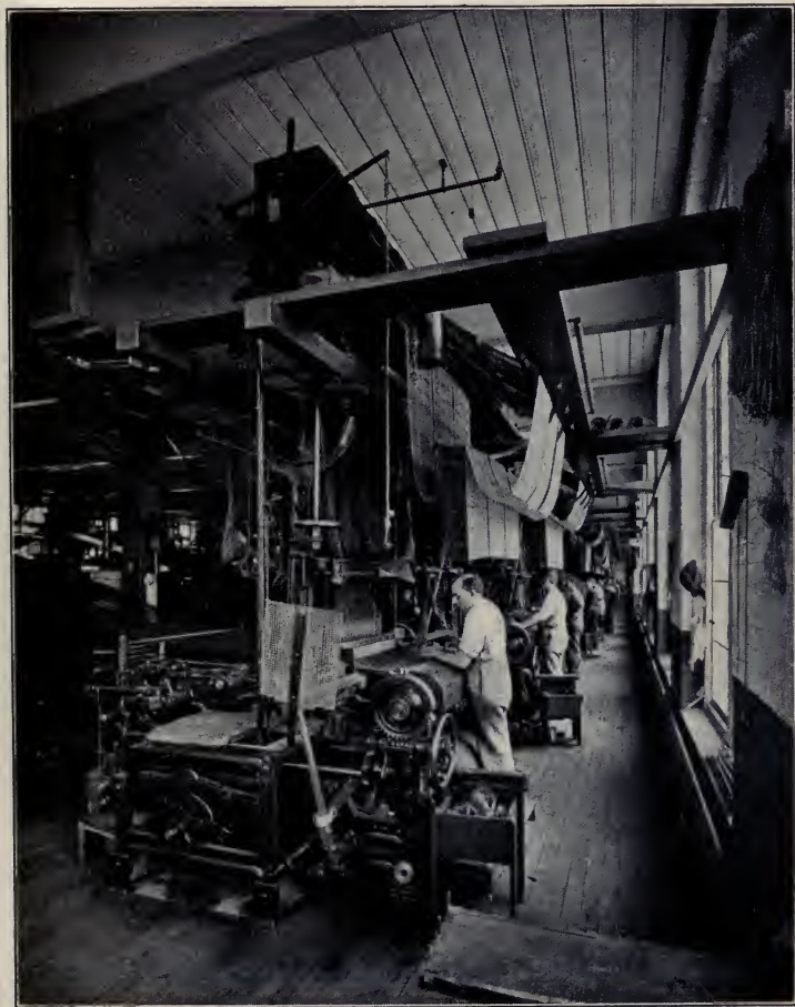
FIG. 73.—This shows the Jacquard loom used for weaving rugs and carpets.
