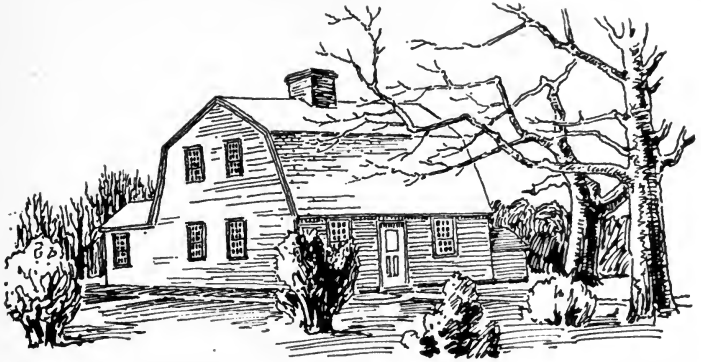
FIG. 7.—A one-storied house with gambrel roof, New England, 18th century. A similar design is used at the present time.
