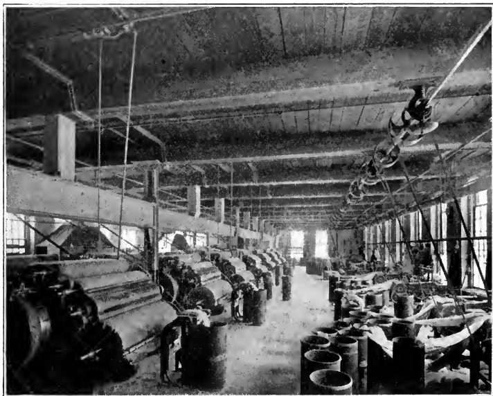
FIG. 67. — Wool carding. Notice the round cylinders revolving around the center cylinder. The web is being delivered into the can at the front.
