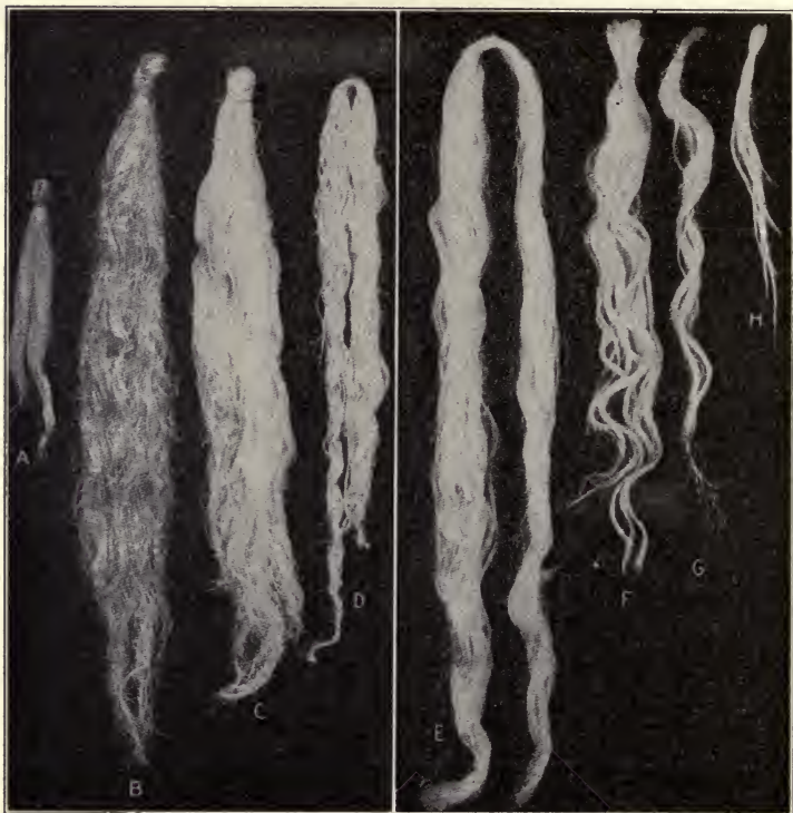
FIG. 63. — Flax and other vegetable fibers used for commercial purposes. [A, Flax; B, C, Hemp; D, Jute; E, F, G, H, Manila, Sisal, and other hard fibers.]
