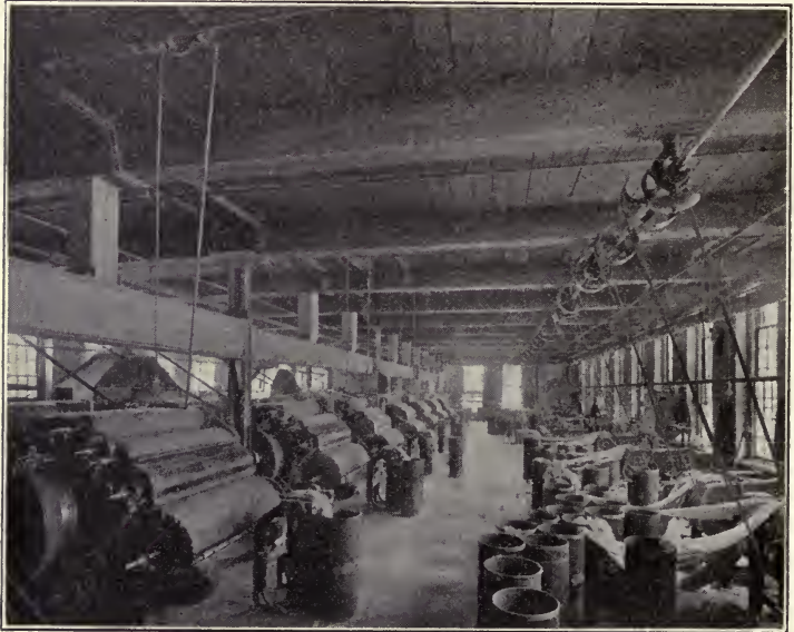
FIG. 67. — Wool carding. Notice the round cylinders revolving around the center cylinder. The web is being delivered into the can at the front.
