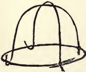
FIG. 146.—Two of the crown wires placed for crown by opposites. Two more to be added.
