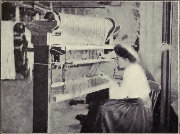
FIG. 49. — Drawing in of threads in preparation for weaving.
