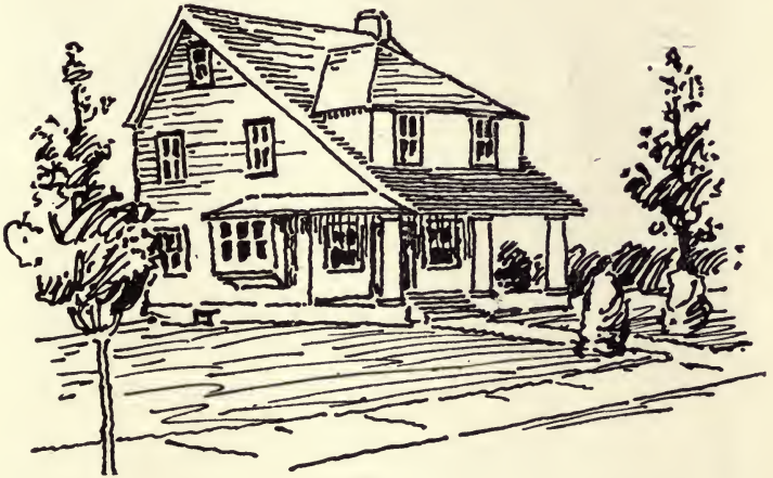
FIG. 9.—A modern small house with the "lean-to" motif. Notice that the long slope faces the front.
