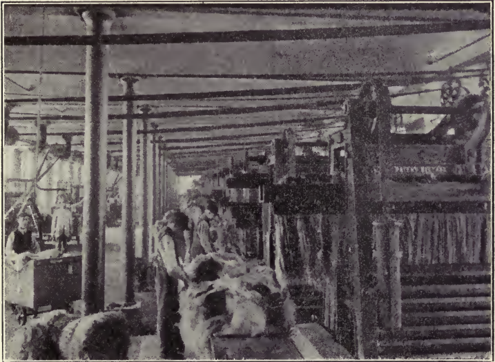
FIG. 53. — Machine hackling or preparation of the flax for the spread boards.
