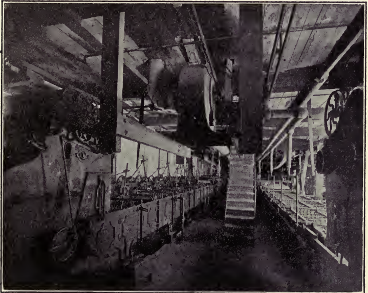
FIG. 66. — Wool washing or scouring. Notice the rakes in the machines which move the wool back and forth in scouring.
