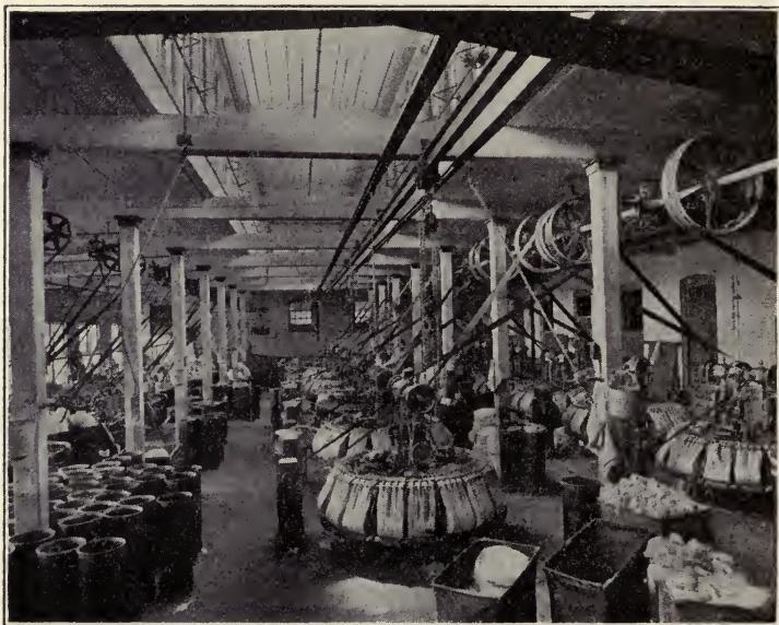
FIG. 68. — Wool combing. This machine is used in the manufacture of high grade wools. There is much waste.
