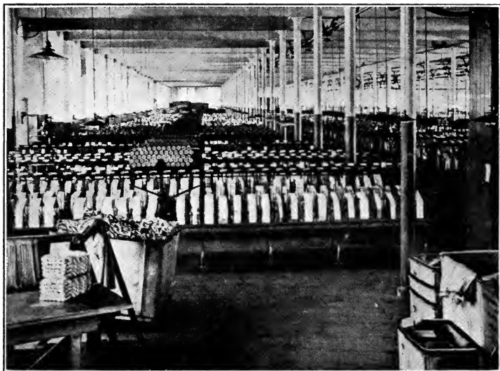
FIG. 82. — Winding room. Silk on swifts.
