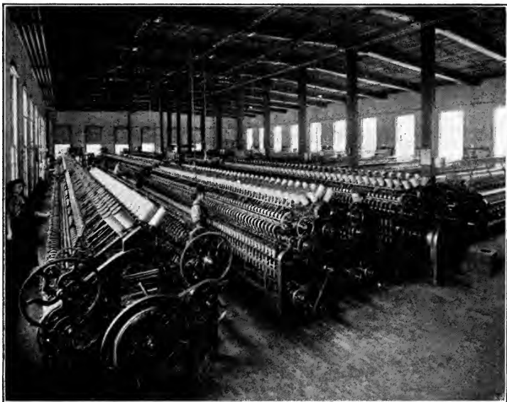
FIG. 72. — This spinning room shows the ring spinning machine in operation.
