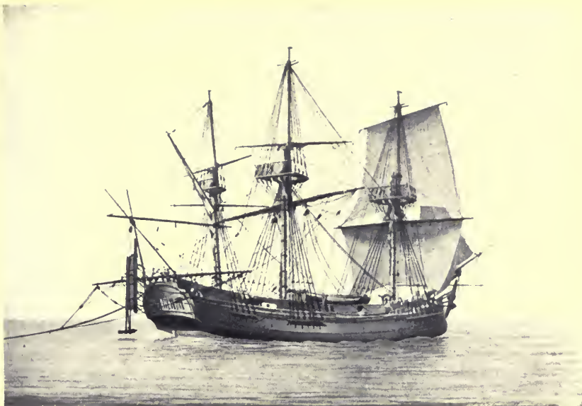
Ship Ulysses —This painting shows a jury rudder about to be put in place at sea, in 1806. So ingenious was the display of seamanship in the rigging of this emergency rudder that her commander, Capt. Wm. Meyford, was awarded a medal by the American Philosophical Society
