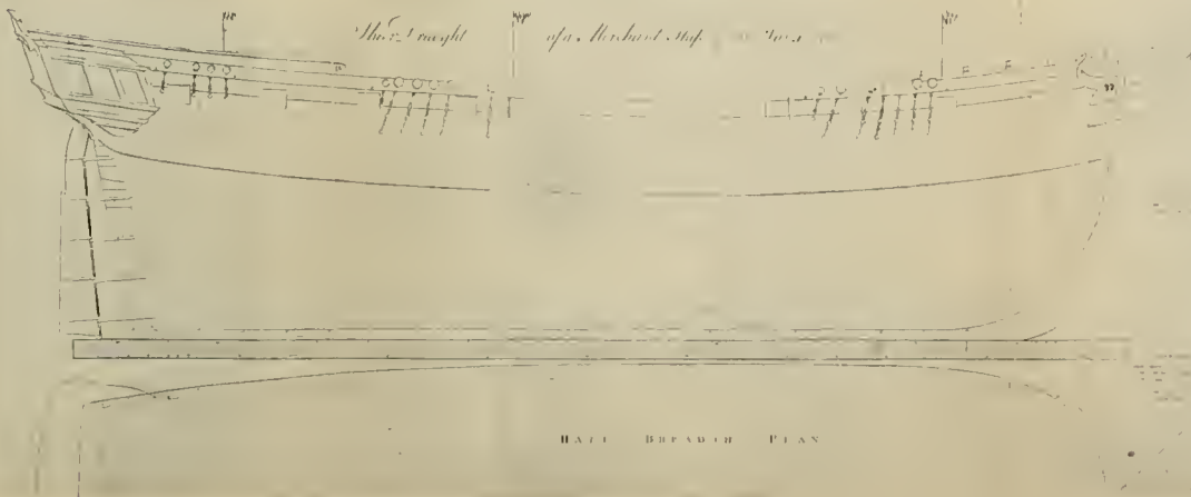
VIII. LONGITUDINAL PLAN OF AN EARLY NINETEENTH-CENTURY 330-TON MERCHANTMAN. Length between perpendiculars, 108 ft. 8 1/2 in. Extreme breadth, 27 ft. 6 in. Depth, 12 ft. Length on keel, 92 ft.
