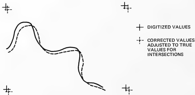
Figure 26. Digitization procedure for correcting shoreline position locations when original shoreline movement map distortions exist
