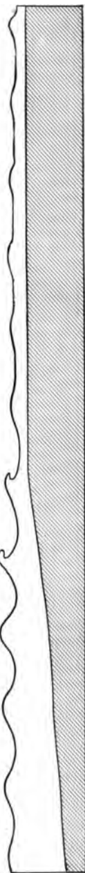
Fig. 7 — Diagram showing how oscillatory waves breaking on a subaqueous terrace produce waves of translation. (After Russell.)
