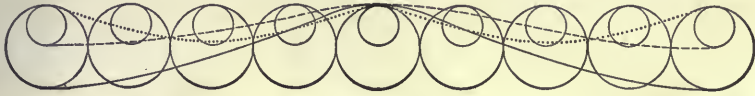
FIG. 4. — Theoretical profiles of three trochoidal waves having different sized orbits (solid-line profile and broken-line profile), or different spacing of orbits (broken-line profile and dotted-line profile). Modified after Grabau.
