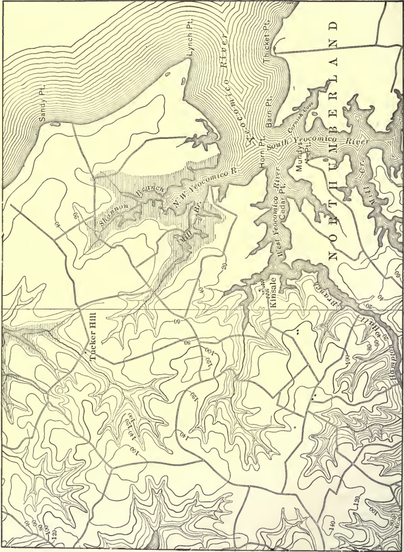
FIG. 46 — Shoreline of submergence in Chesapeake Bay region. Except on the more exposed outer coast the shoreline is not greatly changed from its initial form.
