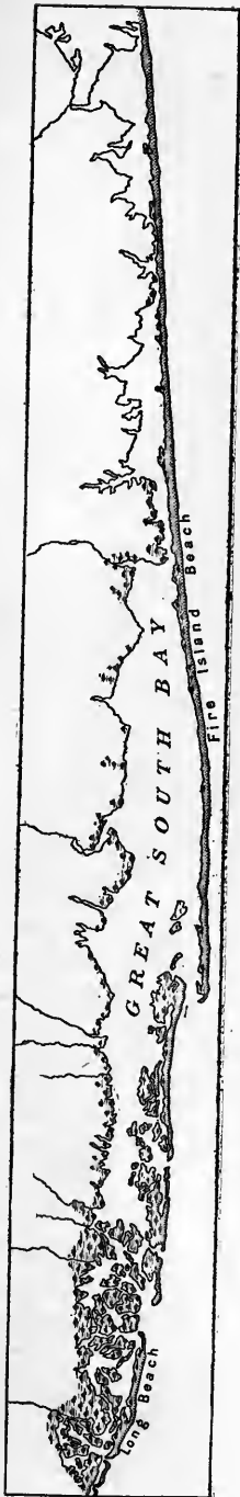
FIG. 115. — Offshore bar and lagoon of the Long Island coast, showing distribution of tidal inlets.
