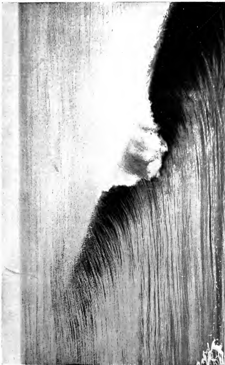
Combing wave, showing water completing orbital movement although insufficient in quantity to fill the wave form.
