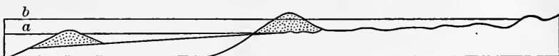
FIG. 44. — Profile of a shoreline of emergence when sealevel is at a , changed to profile of a compound shoreline when submergence brings the sealevel to b and facilitates the landward migration of the offshore bar.
