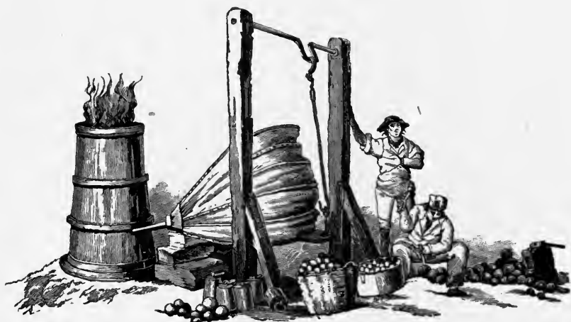
CASTING CANNON BALLS. Pyne, "Microcosm," 1803—1806.
