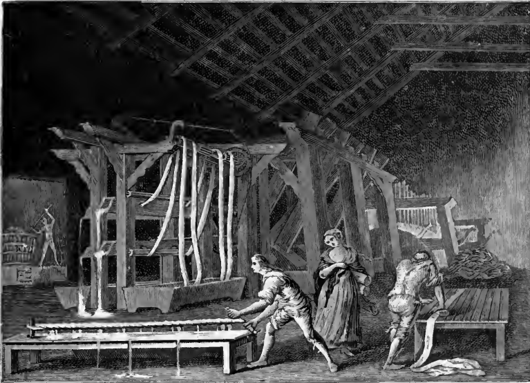
WASH-MILL.—RUBBING BOARDS—BEETLING ENGINE (FOR GLAZING)—BOILING-HOUSE.
