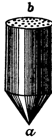
FIG. 6. — THE CLEPSYDRA AS DESCRIBED BY EMPEDOCLES. a , orifice; b , perforated top. Redrawn after Burnet, Early Greek Philosophy , p. 230.
