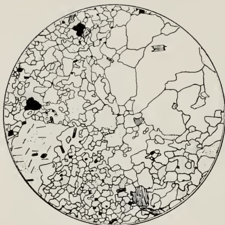
FIG. 3.—Sketch of rhyolite porphyry from Herndon Drilling Co.—Campbell well, Pike County. Clear grains are quartz, stippled are feldspar, black are mostly magnetite and pyrite, and grains with longitudinal lining are biotite and muscovite. Large areas of quartz appear as single grains in plain light. Magnification 48X.
