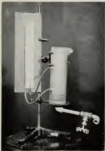
FIG. 2.—Device for measuring permeability of unconsolidated material.
