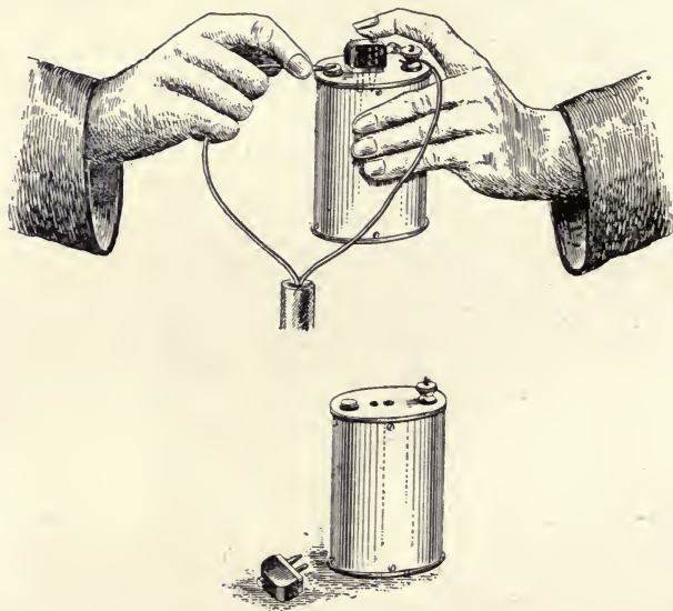
FIG. 48.—DAVIS POCKET SHOT-FIRER, WITH SAFETY KEY.
