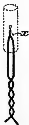
FIG. 53.—SHOWING BRIDGE OF LOW-TENSION FUSE "SHUNTED" BY SHORT-CIRCUITING OF CONNECTING WIRES IN FUSE HEAD.
