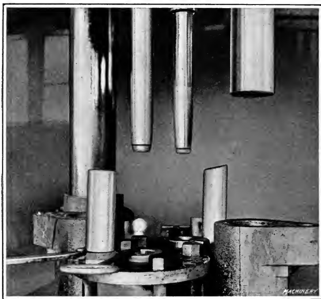
Fig. 8. Drawing Shrapnel Forgings in a "Wood" 750-ton Hydraulic Forging Press
