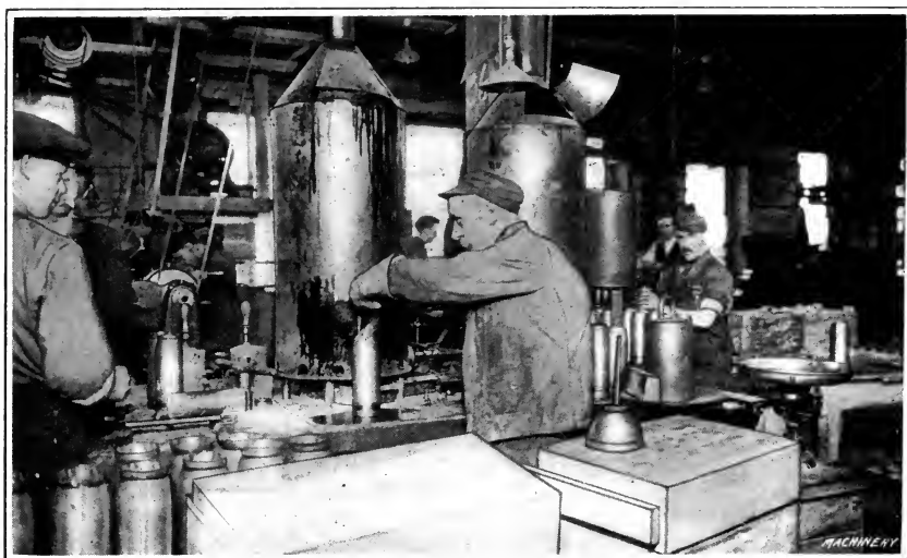
Fig. 22. Assembling Bullets, Resin, and Fuse Socket in Shrapnel Shell
