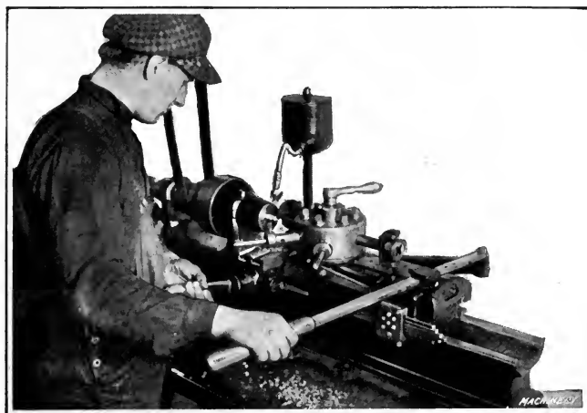
Fig. 19. Machining Fuse Parts on F. E. Wells & Son's Hand Screw Machine
