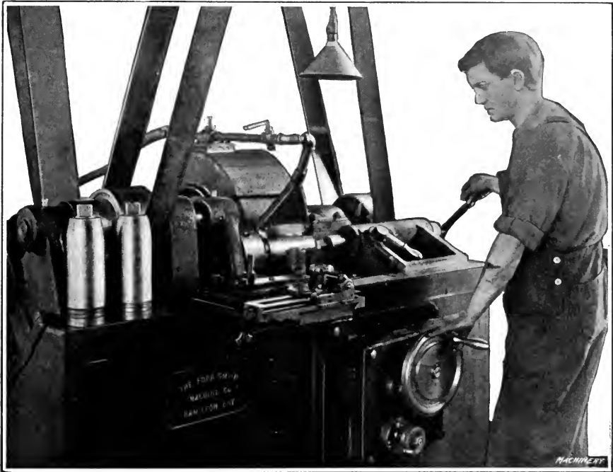
Fig. 17. Grinding Shrapnel Shells in One Operation in a Ford-Smith Grinding Machine carrying a Wheel about 8\frac{1}{4} Inches Wide by 20 Inches in Diameter, rotated at 1200 Revolutions per Minute
