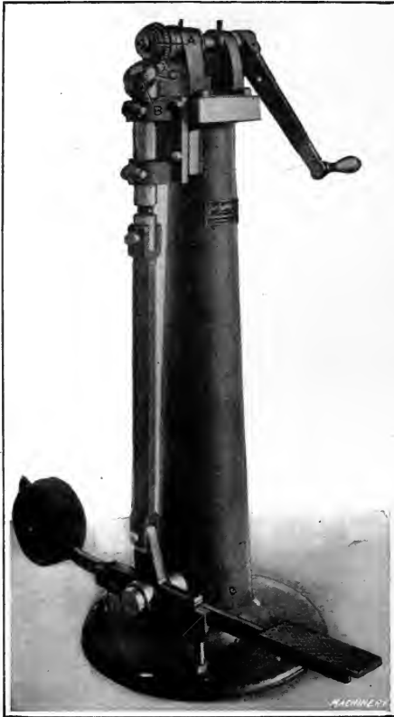
Fig. 22. Graduating Timing Fuse Rings on Dwight-Slate Marking Machine
