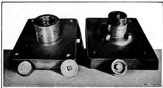
Fig. 3. Tools used for forging Brass Plug
