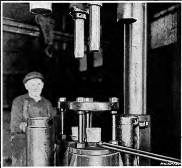
Fig. 7. Piercing Billets for Shrapnel Forgings in a "Wood" 750-ton Hydraulic Forging Press
