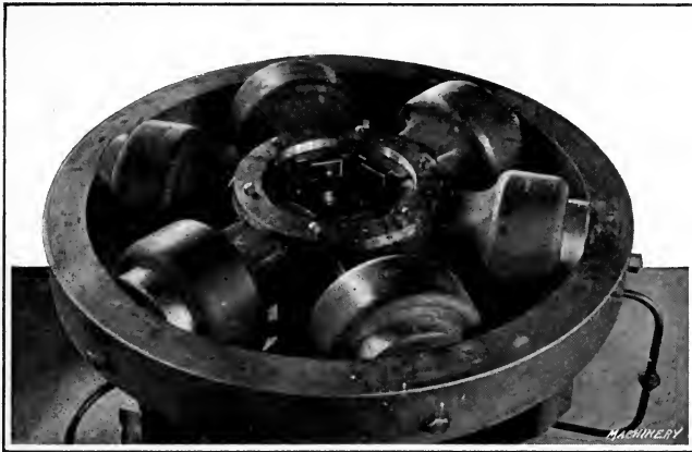
Fig. 20. Close View showing Closing-in Dies of Banding Machine shown in Fig. 18
