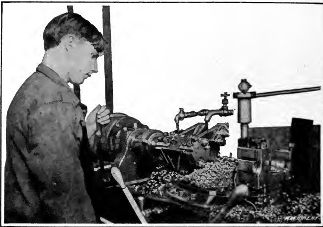
Fig. 6. First Rough-turning Operation on Shrapnel Shell in a Flat Turret Lathe
