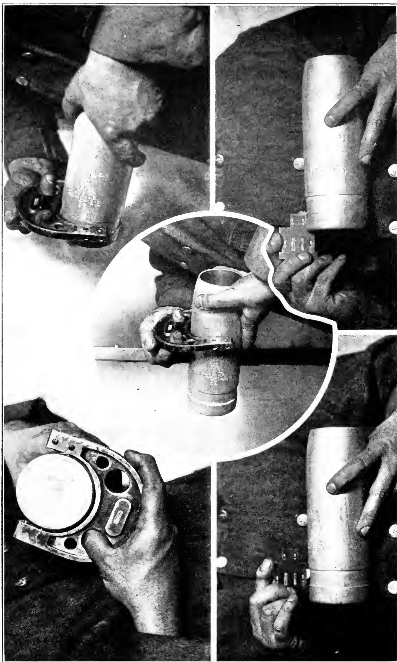
Fig. 24. Illustration showing some of the Principal Gaging Operations on Shrapnel Shells
