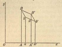
volume, Oa, and pressure, ab, that when, finally, it is compressed in the nonconducting vessel to its original volume OA, it will have regained its original pressure AB, and therefore also its original temperature t. The whole external work done is re-
