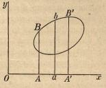
curve whatever from B to B', and so apply heat to the working substance that this curve shall represent the relation of <sup>1</sup> Phil. Trans. 1854. pressure to volume during the expansion, it is evident that the work done cannot generally be expressed in terms of the initial and final conditions of the substance.
