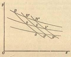
166. Let the co-ordinates of B indicate the pressure and volume of unit of weight of the working substance at the commencement of the experiment; its temperature being  $T_1$ , say that of saturated steam at given pressure.
