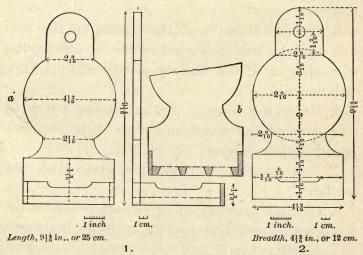
1. Saw out a piece of wood of sufficient size for the back and bottom. Plane face and edge of each at right angles.
