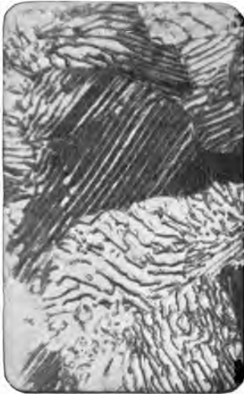
PHOTOMICROGRAPHS SHOWING THE STRUCTURE OF STEEL MADE BY PROFESSOR E. G. MAHIN OF PURDUE UNIVERSITY 1. Cold-worked steel showing ferrite and sorbite (enlarged 500 times) 2. Steel showing pearlite crystals (enlarged 500 times) 3. Structure characteristic of air-cooled steel (enlarged 50 times) 4. The triangular structure characteristic of cast steel showing ferrite and pearlite (enlarged 50 times)
