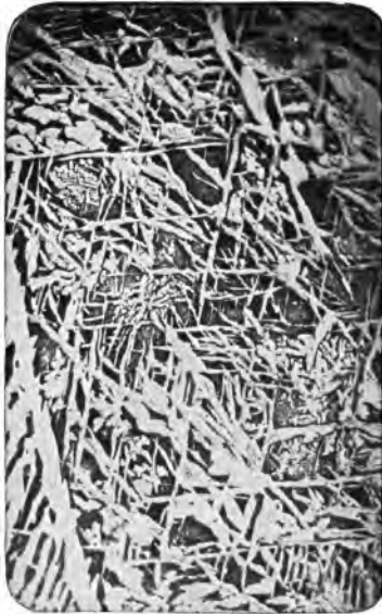
PHOTOMICROGRAPHS SHOWING THE STRUCTURE OF STEEL MADE BY PROFESSOR E. G. MAHIN OF PURDUE UNIVERSITY 1. Cold-worked steel showing ferrite and sorbite (enlarged 500 times) 2. Steel showing pearlite crystals (enlarged 500 times) 3. Structure characteristic of air-cooled steel (enlarged 50 times) 4. The triangular structure characteristic of cast steel showing ferrite and pearlite (enlarged 50 times)
