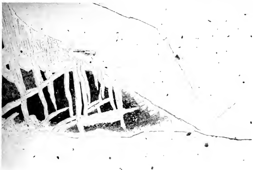
FIG. 1.—A plagioclase field filled with oriented needles characteristic of Kilbourneite . In the upper portion they appear in a ground mass of dense, micro-solved actinolite and epidote ; in the lower portion they are in clear, fully transformed taconite . (Photomicrograph.)
