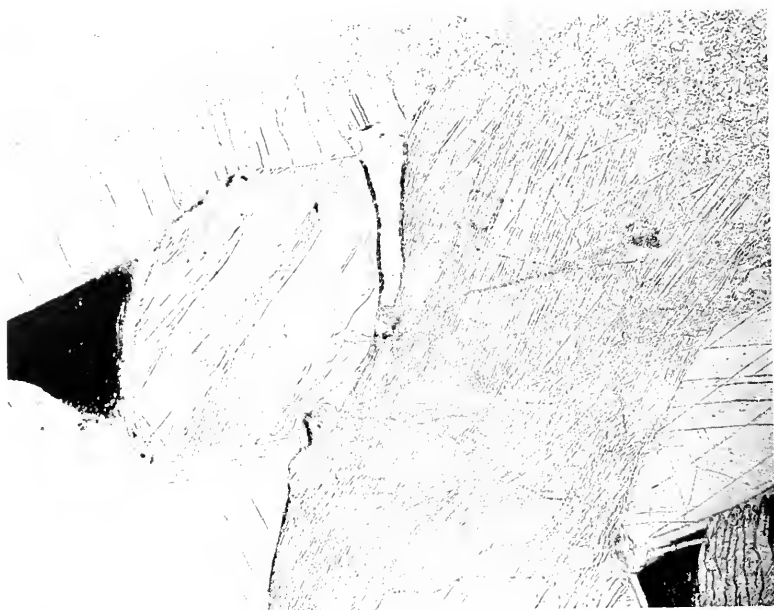
2. An area along the inner border of a zone of alteration at edge of slice. The alteration is apparent along the right-hand side of the photograph. A kamacite band is partly altered, its right-hand boundary having disappeared in the secondary granulation produced by heating during flight through the air. Pictal 120 sec.
