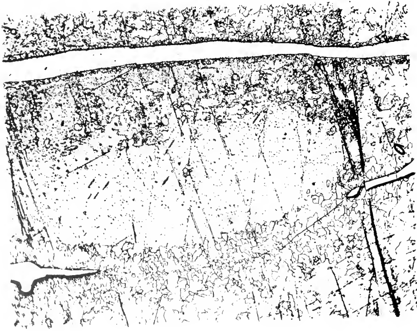
1. GRANULATION IN KAMACITE ALONG LINE CONNECTING TWO SCHREIBERSITE INCLUSIONS.
