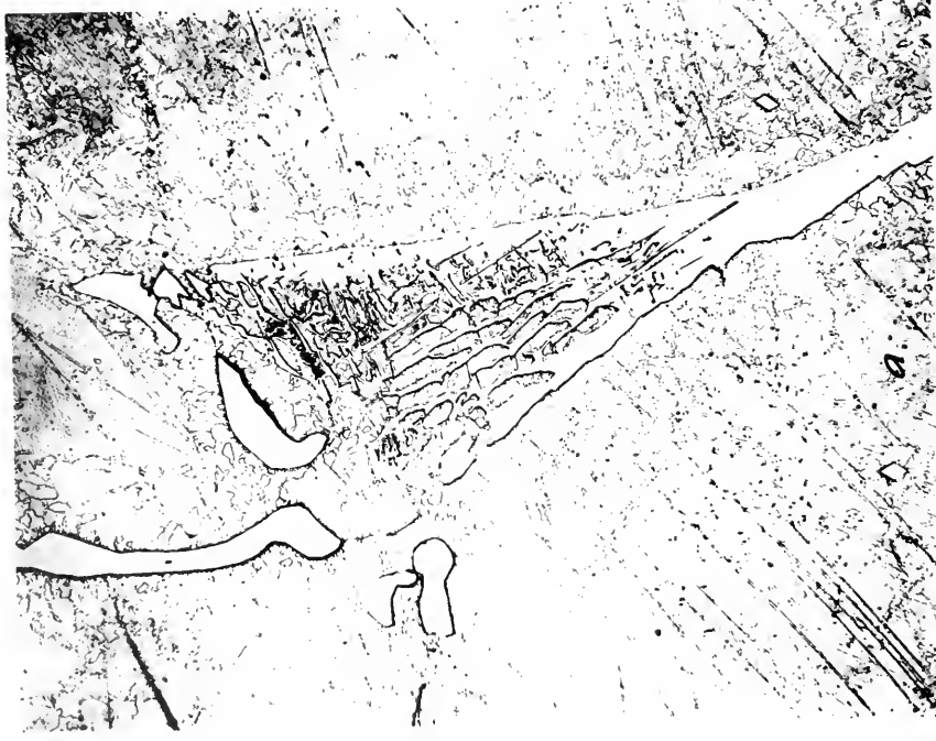
1. WEDGE-SHAPED END OF TAENITE LAMELLA ENCLOSING EUTECTOID PHOSPHIDE AREA Picral, x 100.
