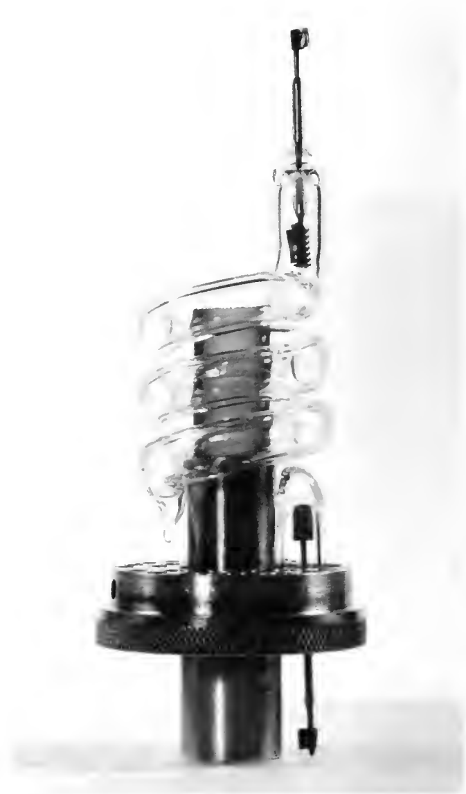
The first laser, constructed by Theodore Maman at Hughes Research Laboratories in 1960, sparked a series of discoveries and applications described in The Laser at 25 , a traveling exhibition organized by the National Museum of Natural History, and produced by the Smithsonian Institution Traveling Exhibition Service in 1985.
