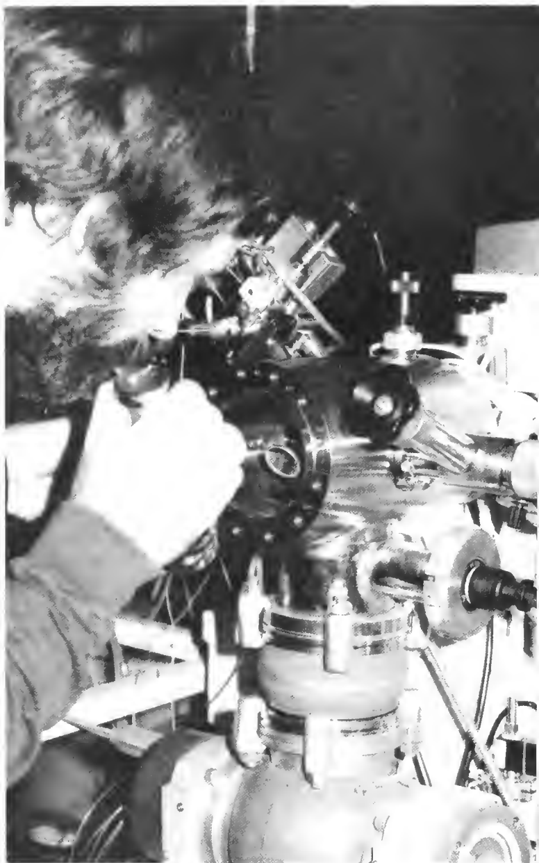
Scientist David Erhardt inspects the port of the Conservation Analytical Laboratory's organic mass spectrometer, which became operational this year. This system is the only one in the United States completely dedicated to research related to museum objects.
