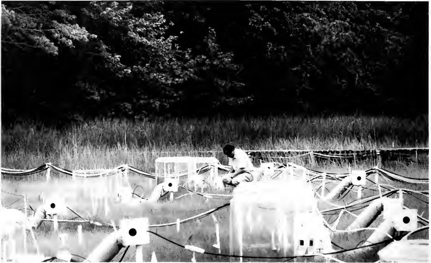
Dr. Bert Drake, plant physiologist at the Smithsonian Environmental Research Center, adjusts controls of an open-top marsh chamber in which carbon dioxide gas concentrations have been doubled to allow measurement of direct and indirect environmental effects.
