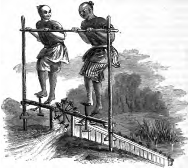
IRRIGATION BY MEANS OF AN ENDLESS CHAIN-PUMP.
