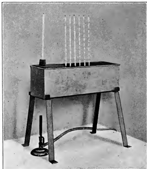
FIG. 5. APPARATUS FOR DETERMINING CONDUCTIVITY OF HEAT
