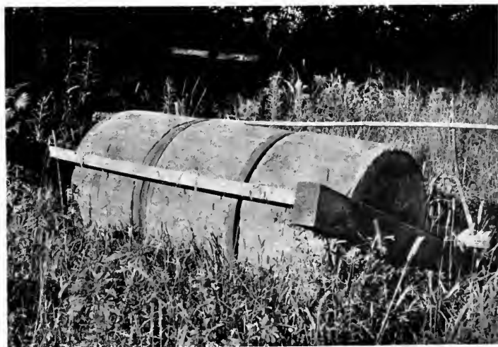
66. A HOME-MADE, THREE-SECTION WOODEN ROLLER
