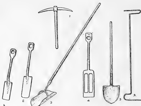
FIG. 66.—Tools for ditching. (1) and (2), ditching spades for removing the major part of the earth from the ditch; (3), grading scoop used to finish the bottom of the ditch and the grade; (4), skeleton spade adapted for use in very plastic soil; (5), shovel for removing loose earth; (6), hook used to place tile in deep, narrow trenches; (7), pick for loosening stone and hard earth.
