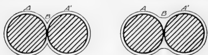
FIG. 32. — Diagram showing the coalescence and readjustment to the capillary film of two soil particles when brought in contact. At left is shown the condition before adjustment with a sharp angle at B ; at right the films are shown in equilibrium with a great thickening at B .
