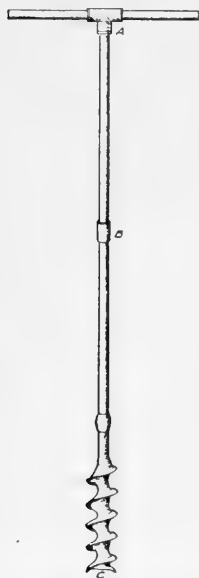
FIG. 83.—Auger used in the examination of soils. (A), handle; (B), joint; (C), worm with modified cutting edge.
